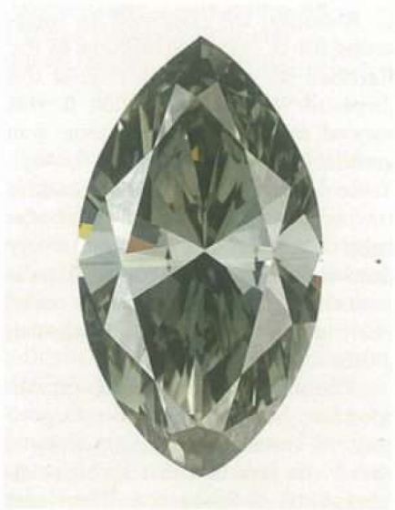
Figure 5. This highly unusual Fancy Dark gray-green diamond (16.54 × 9.13 × 5.87 mm) proved to be type IIb.
